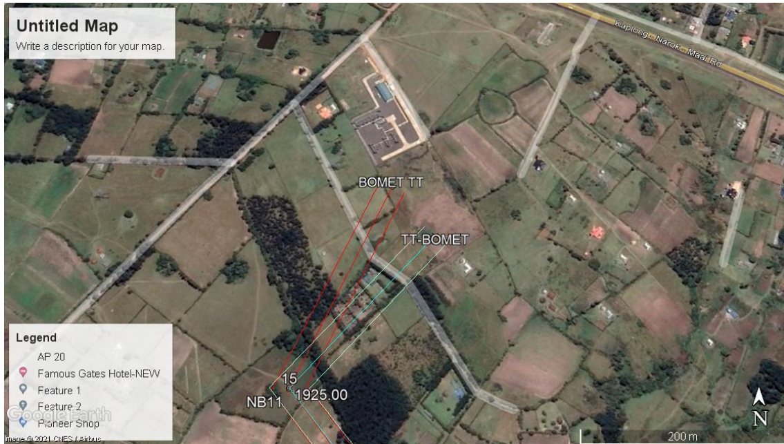
Figure 2-3: Adjustments made at Bomet Substation entry-Red line is KETRACO firm route
