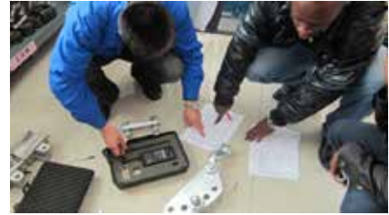
Zinc galvanisation thickness tests
